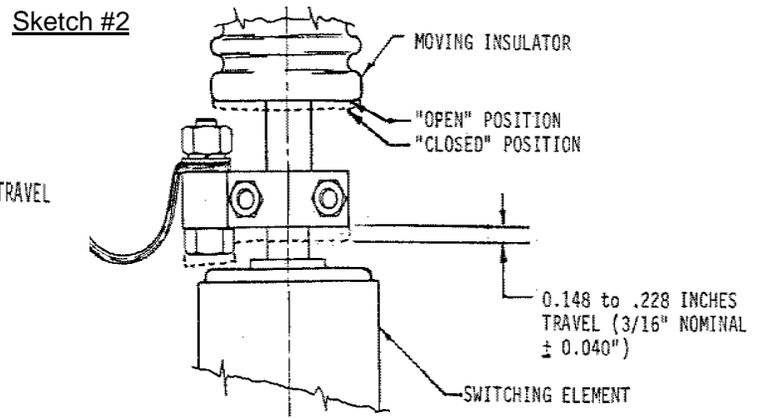
If either of the measurements above is found to be outside of the specified dimensions, vacuum bottle damage or excessive contactor mechanism wear is indicated.
