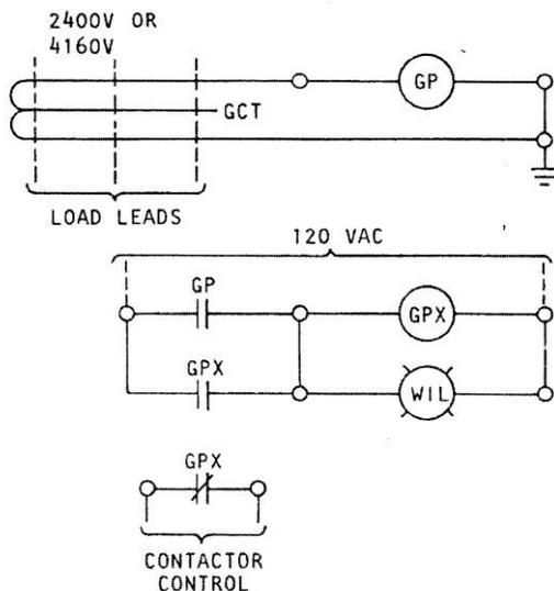
**OPERATION** GP and GCT are coordinated to sense approximately 10-amperes primary ground current (zero-sequence). GP operates instantaneously when this ground current is sensed. As shown in the Schematic Diagram, GPX instantaneously seals-in to energize WIL and to open main contactor. Opening time for opening main contactor is the sum of operating times for GP, GPX, and main contactor. Opening times for Ground Faults of 10-12 amperes or higher, are -
